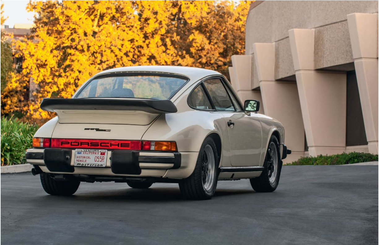
The SCs worldwide rode on 6J x 15 front and 7J x 15 rear wheels with 185/70VR15 front and 215/60VR15 rear tires. The 16s were optional. As noted earlier, power brakes now were standard worldwide. Photo by Randy Leffingwell
