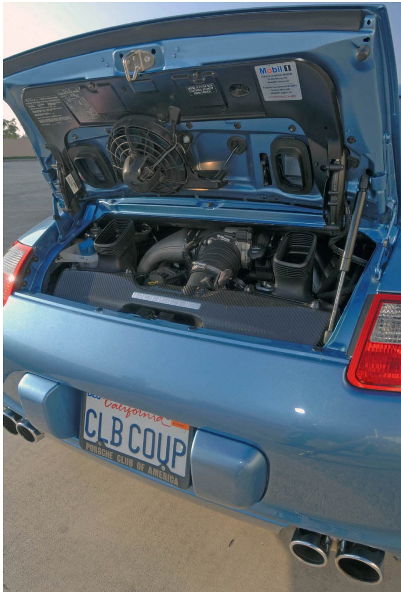
The PCA Coupe was one of the first chances buyers in the United States had access to the desirable X51 Powerkit option for the S engine. Owners described this 26 hp (19 kW) boost—perhaps the wrong word since the engine was definitely naturally aspirated—as a recognizable addition. Photo by Randy Leffingwell
