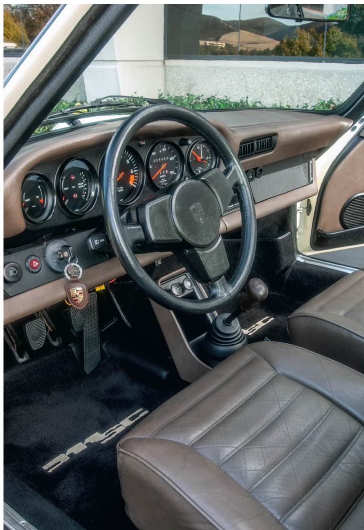
Porsche finished the 1982 SCs with a leather-and-fabric interior. Seat side cushions and the steering wheel were wrapped in the leather. Following two years when US bound cars had speedometers reading only to 85 mph (137 kph), the 150 mph (241 kph) dial returned in 1982. Photo by Randy Leffingwell
