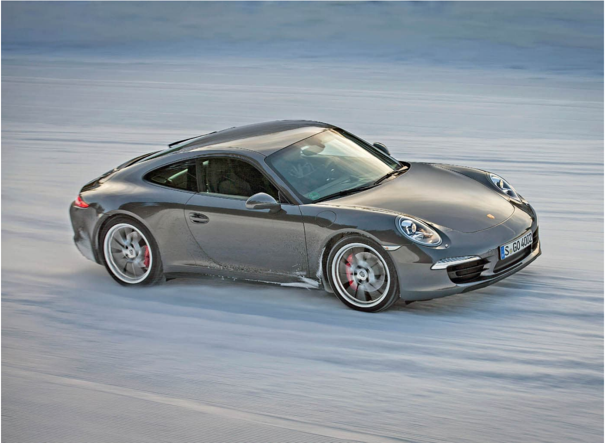
Engineers increased rear track 42 mm (1.7 in) for the 2013 Carrera 4, 4S coupe, and Cabriolet, fitting rear wheels 10 mm (0.4 in) wider than used on 997s. The rear fender bodywork swelled 22 mm (0.9 in) on each side of the C4 models and 36 mm (1.4 in) on each of the 4S rear fenders. Image courtesy of Porsche Press Database
