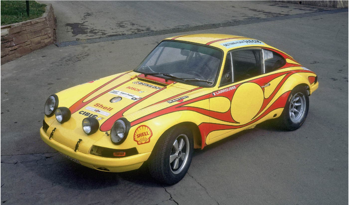
The race shops relied on a 911 S series production floor pan, body structure, and rear fenders, but replaced front fenders, deck lids, doors, and bumpers with fiberglass. Side windows were thinner-gauge plexiglass. It weighed only 789 kg (1,739 lb). Image courtesy of Porsche Corporate Archives
