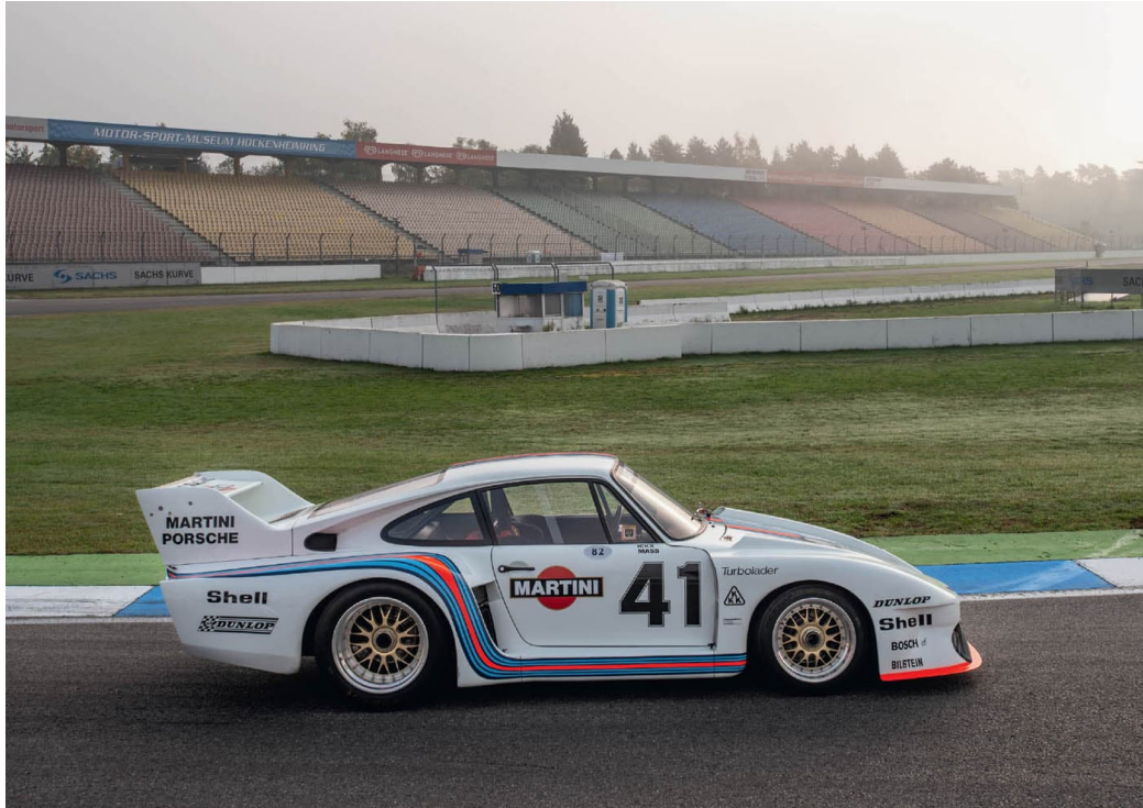
"Baby" was narrower than her sibling, 935-01, the prototype, or all her successors. The full-size 935 relied on 1,558 mm (61 in) rear track, "Baby" circulated on a rear track of 1,457 mm (57 in). This paralleled wheel and tire choices: 19 x 14 inches for 935, compared to 13.5 x 16 inches for "Baby." Photo by Randy Leffingwell
