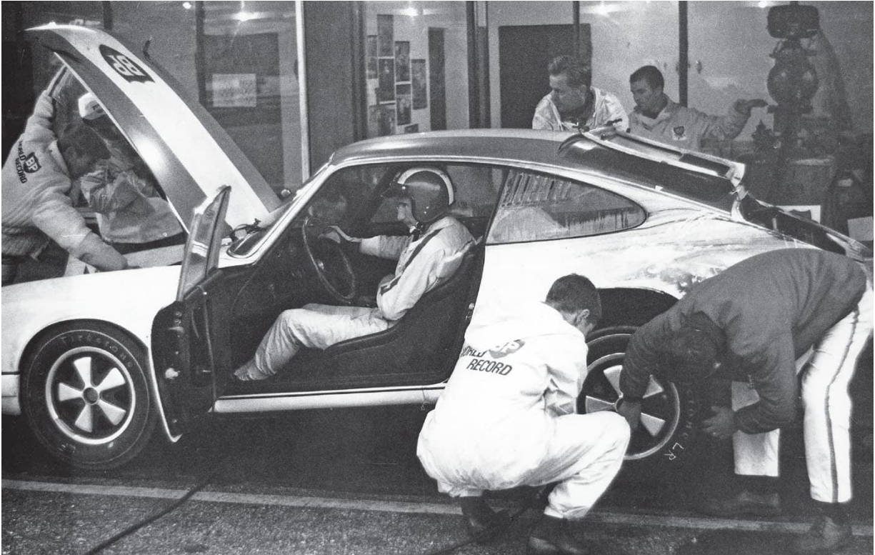
Engineers fitted larger anti-sway bars as well as torsion bars front and rear. Wheel widths grew from 5.5 inches (14.0 cm) to 6.0 inches (15.2 cm) front and 7.0 inches (17.8 cm) in the rear, wearing Dunlop 185 HR 15 racing radials. Here Jo Siffert waited impatiently during a routine tire and wheel change. Image courtesy of Porsche Corporate Archives
