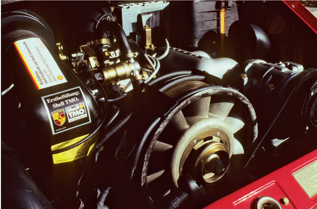
Porsche carried over the 3.2 Carrera engine unchanged for the Speedster. With 3164cc overall displacement, the engine produced 231 hp at 5900 rpm. These Turbolook Speedsters weighed 1290 kg (2,844 lb) and Porsche assembled 2,103. Photo by Randy Leffingwell
