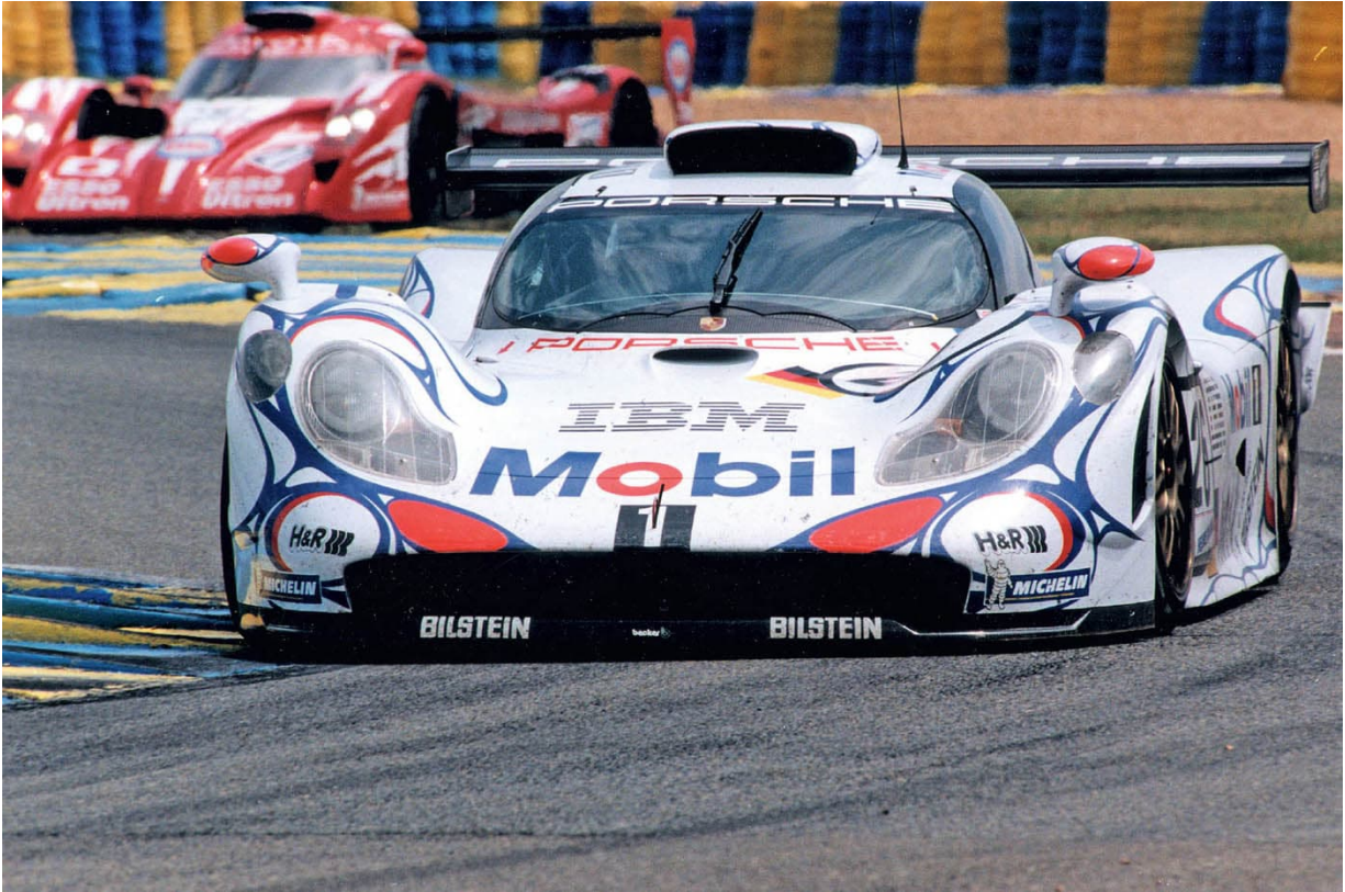
While the car was bigger than the 993 GT1, this new design was superior aerodynamically. New front and rear ends improved down force and did a better job balancing it front-to-rear. Overall, the 1998 GT1 was 100 kg (220 lb) lighter and significantly stiffer than the 1996/1997 versions. Image courtesy of Porsche Corporate Archives
