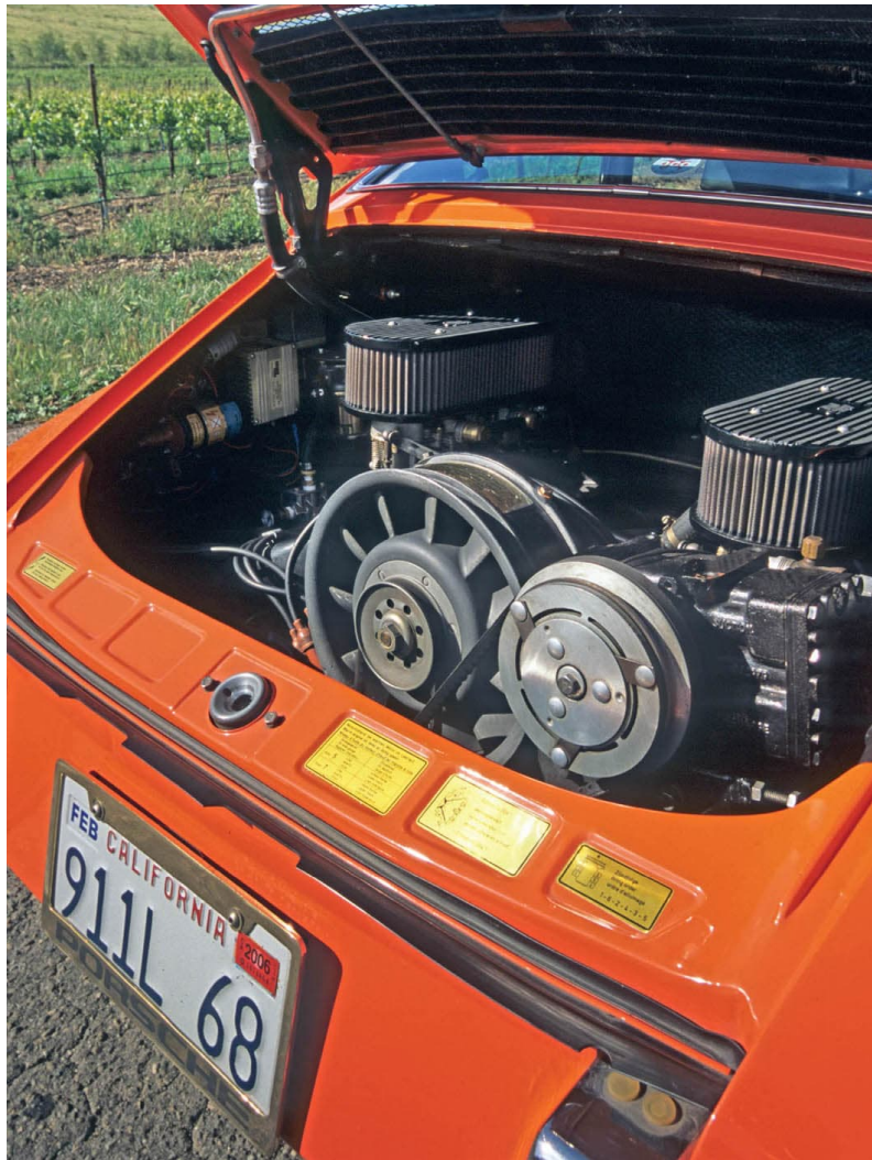
The 1991cc S engine for Europe, Typ 901/02, developed 160 hp (118 kW) at 6600 rpm and produced 132 lb-ft (79 N·m) of torque at 5200 rpm. Unable to get its exhaust clean enough to meet United States emissions standards, Porsche blended the luxury of the S with the platform of the US-legal 130 hp 96 kW) base model and exported it as the 911 L. Photo by Randy Leffingwell
