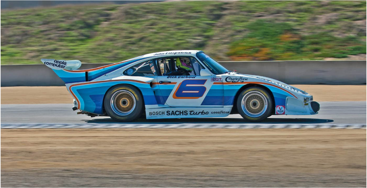
With selected tires and gearing specifically matched for Le Mans, the 935K3s reached top speeds of 350 kph (217 mph) along the Mulsanne Straight. The cars were successful in the DRM and in IMSA in the United States, as with this Dick Barbour team entry. Photo by Randy Leffingwell
